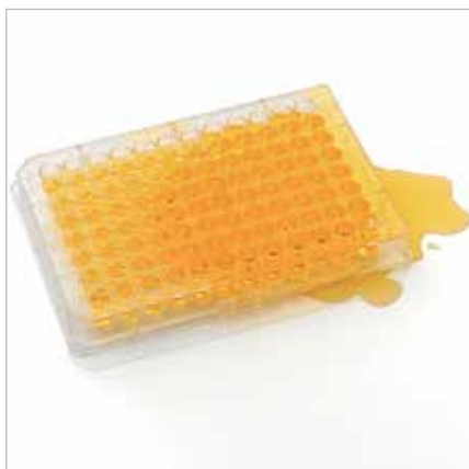
Spilling of plate caused by clogged needles
