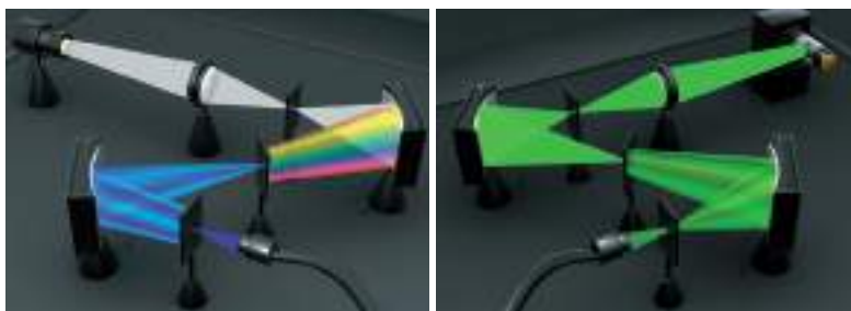
The Quad4 Monochromators technology makes use of a double monochromator on both the excitation and emission side. The picture above outlines the double monochromator system architecture on the excitation (left) and the emission (right picture).
