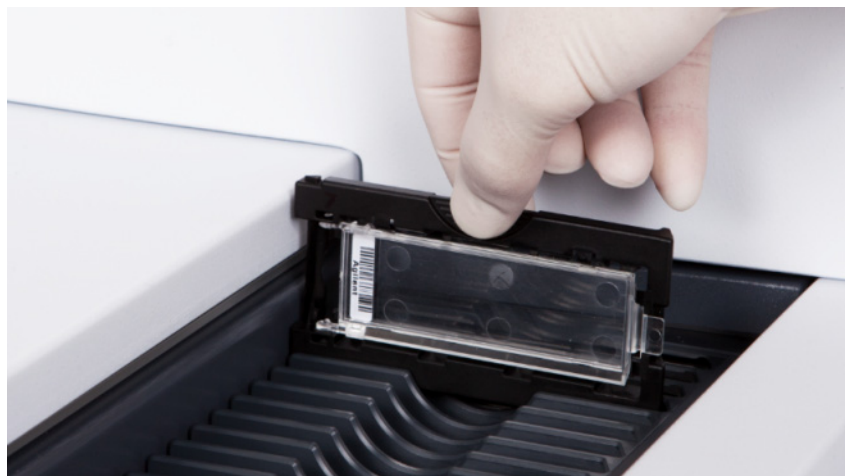
Figure 12 Inserting slide holder into cassette
