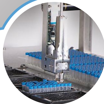
The Universal Picker provides the ability to pick multiple labware types with different diameters in one picker module
