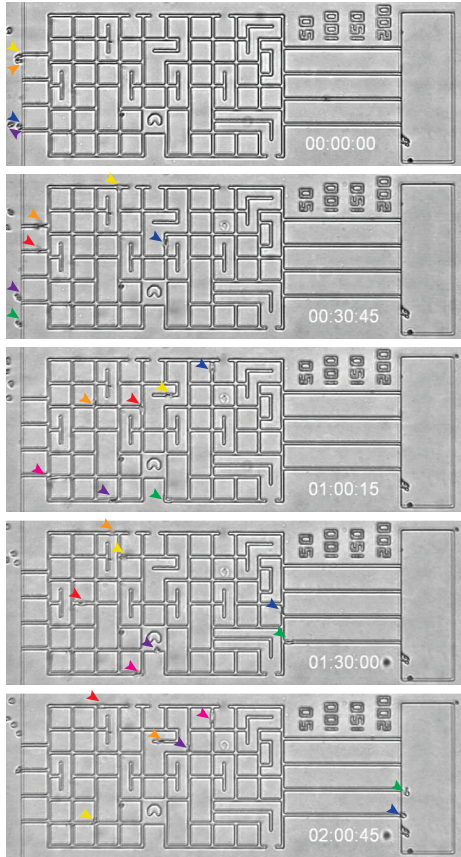
Figure 4. Human neutrophils navigate their way through a microscopic size maze (total maze size is 0.8 mm) towards a reservoir with chemoattractant on the right. Colored arrowheads indicate the same neutrophil at different timepoints. The speed and directionality of neutrophil movement towards the chemoattractant is followed using the CytoSMART™ Lux2.
