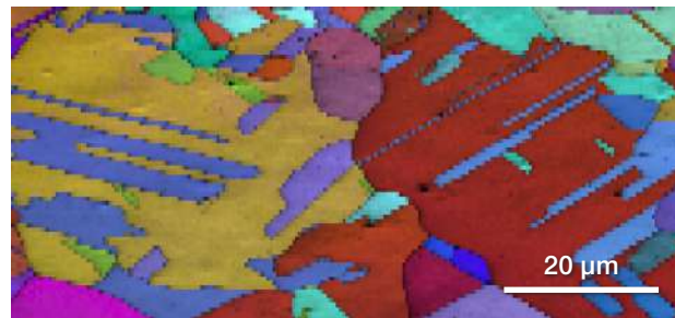
EBSD map of a copper surface. The images show high quality EBSD results even at high temperature.
