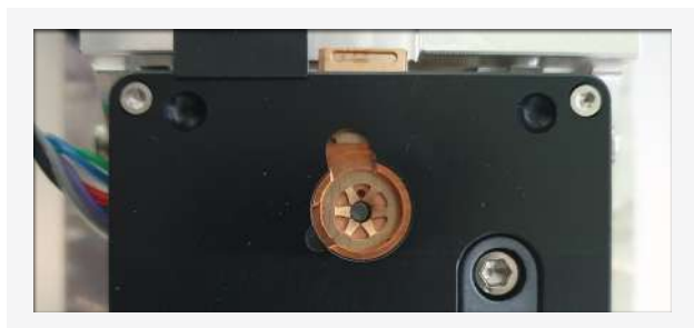
The WetSTEM stage. The hole in the stage allows for humidity-controlled STEM characterization of thin, electron-transparent samples. The stage also functions as a regular cooling stage when a bulk sample is mounted.
