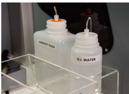
Wash buffer to rinse the strips between the different reagent steps and diluted ethanol solution to accelerate the drying step.
