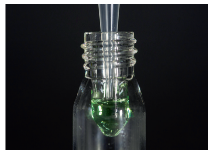
Barometric sensor detects atmospheric pressure changes for level sensing of samples and reagents.
